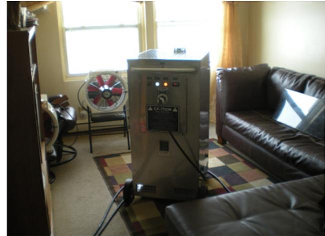
Process involves heating unit over 130 degree F using thermal heater or steaming over 120 degree F preferably with dry vapor steamer
